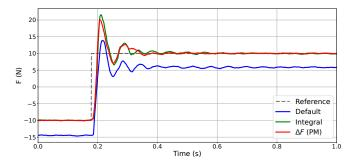
Fig. 3: Lateral force trajectories in the  $e_x$  direction for the force step tracking task: the blue curve is the classical MPC (Default), the green curve is the classical MPC with with integral control (Integral) and the red curve is the force offset estimation  $\Delta F$  included in the predictive model ( $\Delta F$  (PM)).
