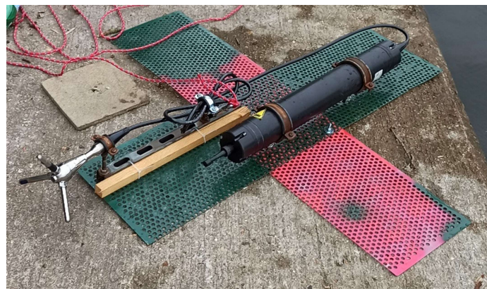
Figure S3. Side-looking ADV positioning frame used for the Mass Transfer Coefficient (MTC) method
