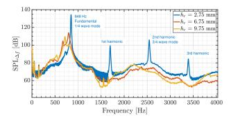
**FIGURE 10**: Spectral distribution of Sound Pressure Level obtained with constant chamber length  $l_c = 165$  mm and S = 0.60 for the unstable operating point 2 presented in Fig. 6: thermal power  $\mathcal{P}_{th} = 1.62$  kW and global equivalence ratio  $\phi = 0.42$ . Three values for the recess length  $h_r$  are presented: 2.75 mm, 6.75 mm and 9.75 mm.
