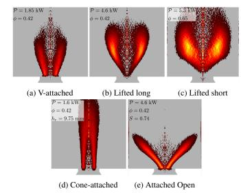
**FIGURE 3**: Abel-deconvoluted OH\* chemiluminescence images of different flame shapes observed with the tube length  $l_c=150$  mm. The swirl number is (a,b,c,d) S=0.60 and (e) S=0.74. The recess length is (a,b,c,e)  $h_r=6.75$  mm and (d)  $h_r=9.75$  mm. The global equivalence ratio is (a,b,d,e)  $\phi=0.42$  and (c)  $\phi=0.65$ . The thermal power is (a)  $\mathcal{P}_{th}=1.85$  kW, (b,e)  $\mathcal{P}_{th}=4.6$  kW, (c)  $\mathcal{P}_{th}=5.3$  kW and (d)  $\mathcal{P}_{th}=1.6$  kW.
