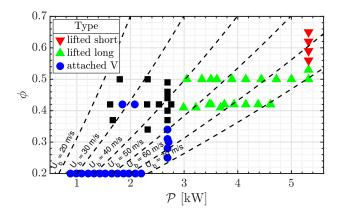
**FIGURE 5**: Types of flame shapes obtained with the baseline geometry: S = 0.60,  $h_r = 6.75$  mm and  $l_c = 150$  mm, as a function of thermal power  $\mathcal{P}_{th}$  and global equivalence ratio  $\phi$ . The black squares correspond to unstable points for this geometry. Dashed lines represent iso-bulk velocities of the fresh gases.
