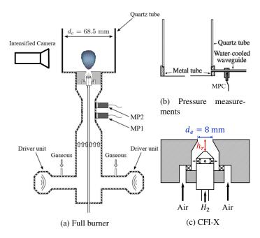
**FIGURE 1**: Experimental setup, adapted from [18]: full burner for (a) flame visualization, (b) pressure measurements, and (c) CFI-X with atomizer replaced by the crossflow injection head.
