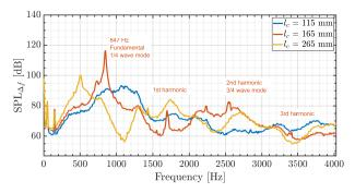
**FIGURE 11**: Spectral distribution of Sound Pressure Level obtained with constant recess length  $h_r = 6.75$  mm and S = 0.60 for the unstable operating point 3 presented in Fig. 9: thermal power  $\mathcal{P}_{th} = 2.31$  kW and global equivalence ratio  $\phi = 0.42$ . Three values for the quartz tube length  $l_c$  are presented: 115 mm, 165 mm and 265 mm.
