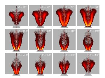
**FIGURE 9**: Phase averaged OH\* chemiluminescence images of the unstable flame at  $\mathcal{P}_{th}=2.31$  kW and  $\phi=0.42$  (Point 3), obtained with the baseline geometry: S=0.60,  $h_r=6.75$  mm and  $l_c=150$  mm. The phase angle is denoted by  $\theta$ .
