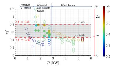
**FIGURE 12**: Values of the time delay between the CFI-X and the flame barycenter for all the operating points used with all geometrical configurations. The filled circles are unstable flames, while unfilled circles are used for stable flames.
