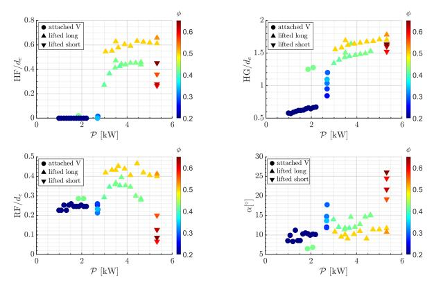
**FIGURE 4**: Evolution of the four metrics HF (foot height), HG (height of the barycenter), RF (foot radial position) and  $\alpha$  (opening angle) as a function of thermal power  $\mathcal{P}_{th}$  and global equivalence ratio  $\phi$ , for all the operating points used with baseline geometry parameters: S = 0.60,  $h_r = 6.75$  mm and  $l_c = 150$  mm.
