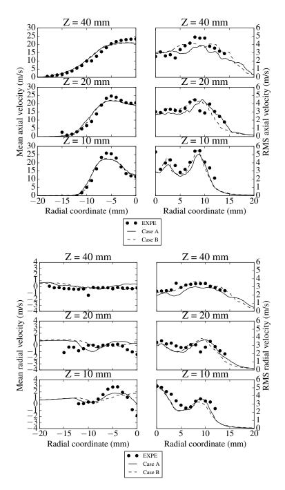
Fig. 3 Cold case mean and RMS gas axial (top) and radial (bottom) velocity. Symbols: experiments, solid line: Case A, dashed line: Case B.
