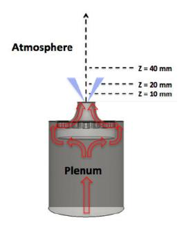
Fig. 1 Experimental setup. Air path in red, spray injection in blue. From [4].
