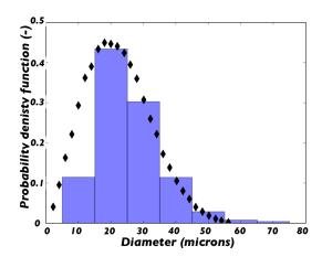
Fig. 2 Particle size distribution. Experiments: blue bars, Rosin-Rammler distribution: black diamonds.
