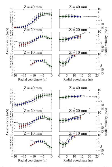
Fig. 6 Cold case (top) and reacting case (bottom) mean axial (left column) and radial (right column) spray velocity. Symbols: experiments (green:  $d_p < 15$  mm, blue:  $15 < d_p < 35$  mm, red:  $35 < d_p$  mm), solid line: Case A, dashed line: Case B.
