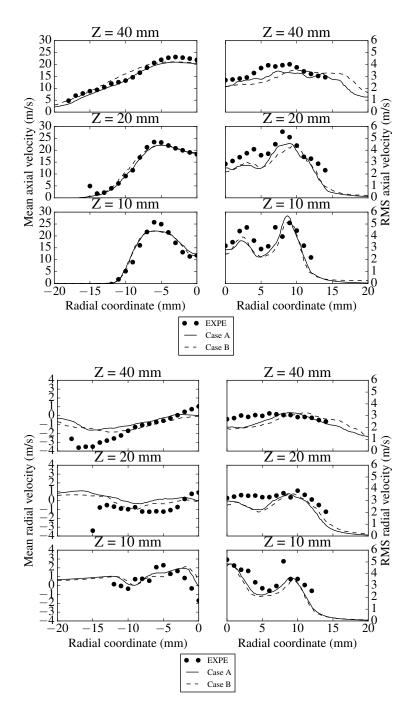
Fig. 4 Reacting case mean and RMS gas axial (top) and radial (bottom) velocity. Symbols: experiments, solid line: Case A, dashed line: Case B.
