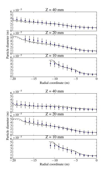
Fig. 5 Cold case (top) and reacting case (bottom) mean spray diameter. Symbols: experiments, solid line: Case A, dashed line: Case B.
