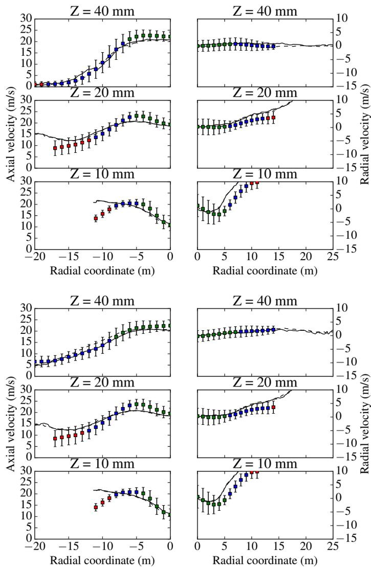
Fig. 6 Cold case (top) and reacting case (bottom) mean axial (left column) and radial (right column) spray velocity. Symbols: experiments (green:  $d_p < 15$  mm, blue:  $15 < d_p < 35$  mm, red:  $35 < d_p < 60$  mm), solid line: Case A, dashed line: Case B.
