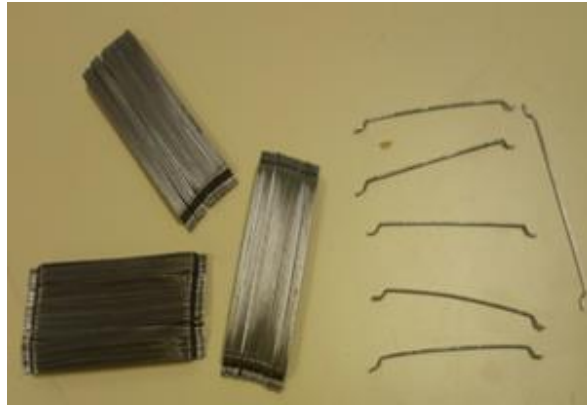
Figure 2. Fibres with end hooks.
