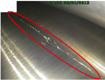
Figure 2. Cracked inner race of the high speed shaft bearing after the last day of recording.
