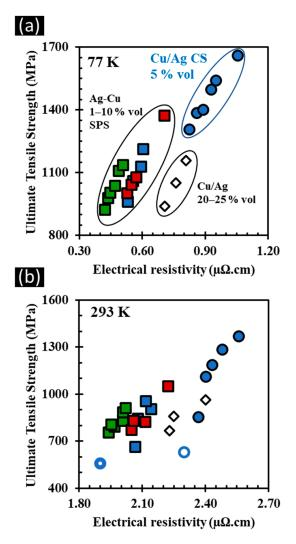
**Figure 14.** UTS vs. electrical resistivity at 77 K (**a**) and 293 K (**b**) for the present Cu/5Ag CS-alloyed wires (**•**) and bulk *CS* as-deposited (**•**) and heat-treated (**•**) SPS composite Ag-Cu (1, 5, and 10 vol. % Ag) wires (**•**, **•**, **•**) [10] and alloyed Cu/Ag (21–25 vol. % Ag) wires (**\$•**) [4–6].
