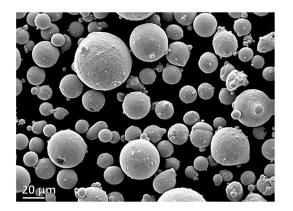
Figure 2. SEM image of the Cu/5Ag powder particles.
