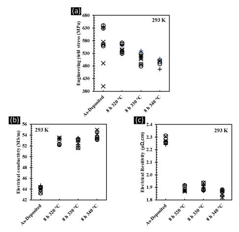
**Figure 9.** (a) Engineering yield strength, (b) electrical conductivity, and (c) electrical resistivity measured at 293 K of the as-deposited and heat-treated Cu/5Ag samples in radial (**x**), tangential (**+**), and longitudinal (**O**) directions.
