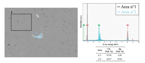
**Figure 4.** SEM image and corresponding EDS spectra of the CS deposit. The black (1) and blue (2) areas indicate the EDS analysis areas.
