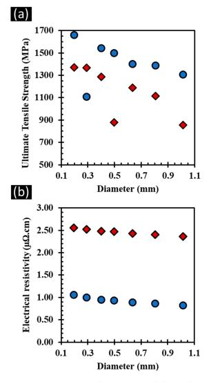
**Figure 13.** UTS vs. wire diameter (**a**) and electrical resistivity vs. wire diameter (**b**) at 293 K (◆) and 77 K (●) for present wires.
