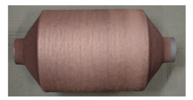
Figure 1. Photograph of the Cu/5Ag CS deposit.
