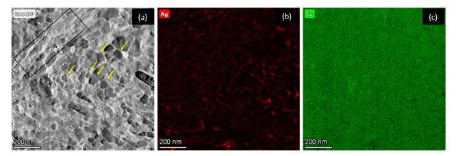
**Figure 6.** STEM HAADF image (**a**) and STEM-EDS Ag mapping (**b**) and Cu mapping (**c**) of the transversal section of wire ( $\emptyset = 0.5$  mm). The yellow arrows indicate regions with nearly equiaxed grains and the black rectangle indicates regions with elongated ribbon-like grains.
