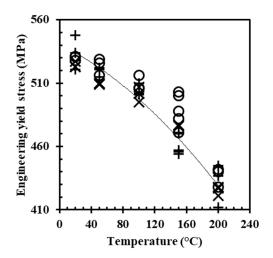
**Figure 10.** Evolution of engineering yield strength in radial (X), tangential (+), and longitudinal (O) directions with temperature for the Cu/5Ag CS-deposited material with an 8 h heat treatment at 330 °C.
