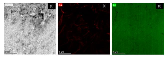
Figure 5. STEM HAADF image (a) and STEM-EDS elemental mappings (b,c) of the CS deposit.
