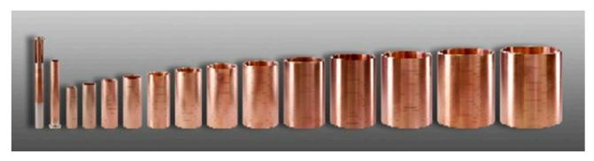
**Figure 8.** Helices (tubes cut helicoidally) for steady-field production. The outer diameter of the largest tube (right) is 372 mm. The weight of the powder necessary for the corresponding deposit before final machining is 120 kg. Today, all tubes are prepared using the CS bulk deposit process.
