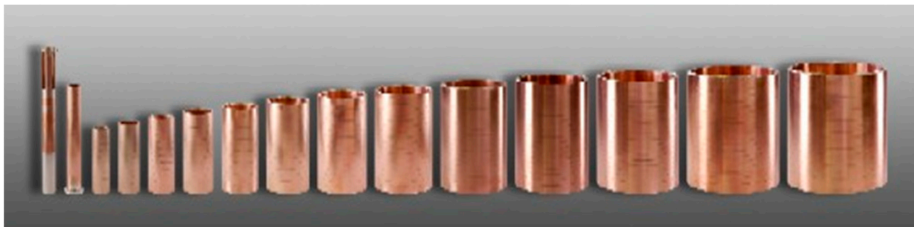
Figure 8. Helices (tubes cut helicoidally) for steady-field production. The outer diameter of the largest tube (right) is 372 mm. The weight of the powder necessary for the corresponding deposit before final machining is 120 kg. Today, all tubes are prepared using the CS bulk deposit process.
