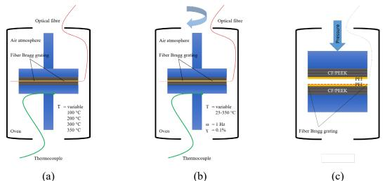
Figure 1. Experimental set-up of rheometer procedure in (a) static mode (b) dynamic mode (c) zoom of assembly
