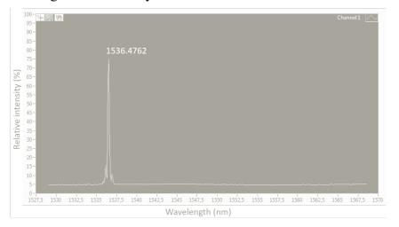
Figure 2. Amplitude reflection coefficient of FBG
