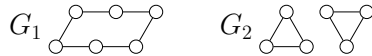
Figure 1: Two non-isomorphic graphs G_1 (6-cycle) and G_2 (two disjoint 3-cycles) which the WL algorithm returns the same outputs, thus failing to distinguishing them.
