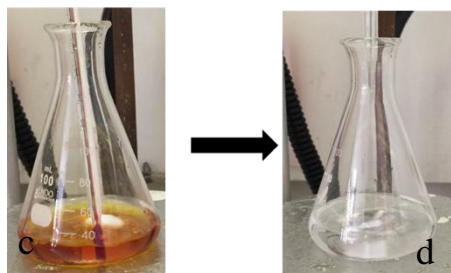
Figure 3: Pictures representing the different states of colorimetric titration (before the equivalence volume (a, c) and after (b,d) of iodine using an aqueous solution of Na 2 S 2 O 3 and using TPP.
