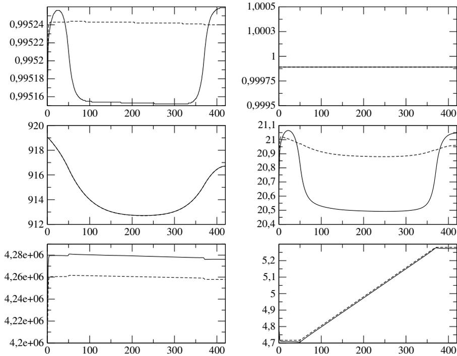
**Figure 6. Heated pipe without any mass transfer: profiles along the main axis of:  $\alpha_l$  (top left),  $m_l/(m_l + m_v)$  (top right),  $\rho_l$  (medium left),  $\rho_v$  (medium right),  $P_l$  (bottom left),  $U_l$  (bottom right), at time  $T = 5$ . Plain line: weak interphase heat transfer ( $\tau_4 = 10^{-1}$ ), dashed line: high interphase heat transfer ( $\tau_4 = 10^{-5}$ ).**
