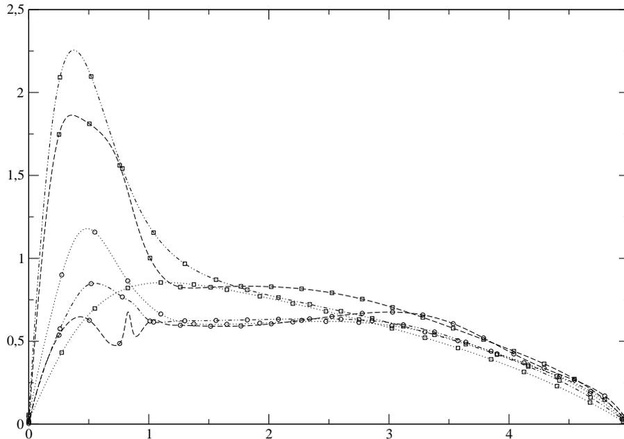
Figure 5. Stratified layer: relative Mach number  $(U_v - U_l)/c_l$  at different times  $T = 0.004$  (dotted line),  $T = 0.01$  (dotted-dashed line),  $T = 0.05$  (dashed line). Circles: with mass transfer, squares: without mass transfer.
