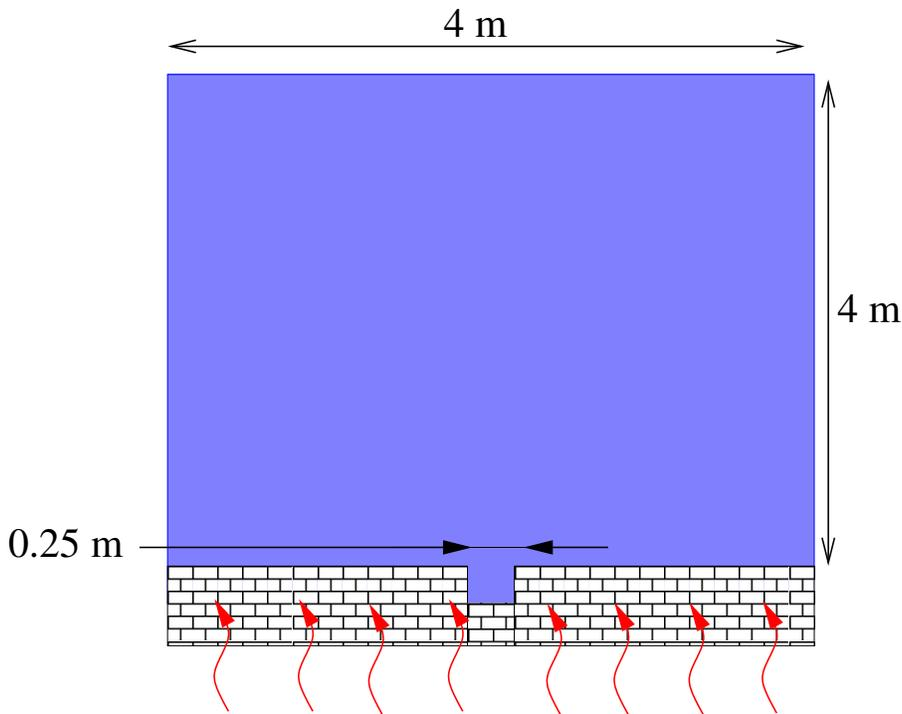
Figure 1. Heated wall: sketch of the computational domain
