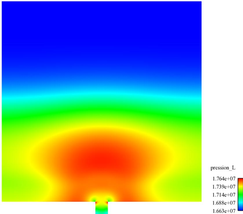
Figure 3. Heated wall: contours of the liquid pressure  $P_l$  at time  $T = 0.0237$ .
