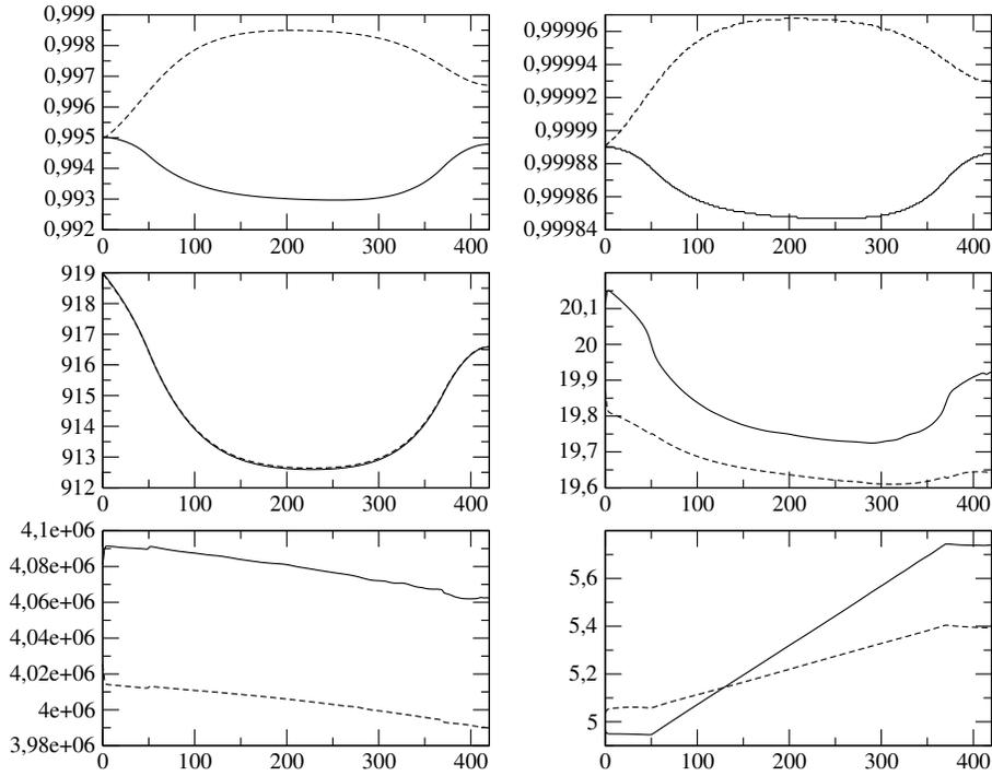
Figure 7. Heated pipe with mass transfer: profiles along the main axis of:  $\alpha_l$  (top left),  $m_l/(m_l + m_v)$  (top right),  $\rho_l$  (medium left),  $\rho_v$  (medium right),  $P_l$  (bottom left),  $U_l$  (bottom right), at time  $T = 5$ . Plain line: weak interphase heat transfer ( $\tau_4 = 10^{-1}$ ), dashed line: high interphase heat transfer ( $\tau_4 = 10^{-5}$ ).
