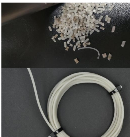
Fig. 10. Samples of as-formed (left) and on-line pelletized (right) extruded filament of the PE-1:4:0.2 composition. At this stage, the compound is in its thermolatent pre-vitrimer form.
