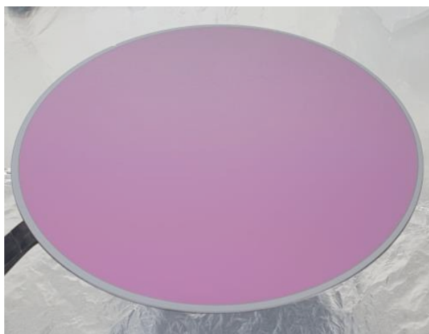
Figure 2. GaN-based heterostructure for integrated photonics grown by molecular beam epitaxy with a Riber R49 reactor on a Si 200 mm diameter substrate. The uniform color indicates an excellent thickness uniformity (below \pm 1\% ). The surface roughness (rms) is 0.7 nm.
