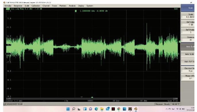
Fig. 5 (a) Wireless setup consisting of a computer controlling a network analyzer, with port 1 connected to a directional antenna. In front of this antenna is the resonant cavity and its antenna, which modulates the reflection of the RF signal based on the measurement of the audio signal captured by the cavity membrane. (b) Visualization of the signal in Zero Span mode (a function of the VNA that can be interpreted as amplitude demodulation).
