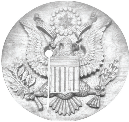
Fig.2. Replica of the Great Seal of the United States of America (56 cm in diameter) with the location of the spy microphone (23 cm long), commonly referred to as "The Thing," "The Great Seal Bug," or "Endovibrator"
