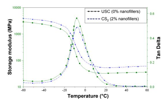
**Figure 10.** Viscoelastic properties of crude polymer (UCS) and CS<sub>2</sub> nanocomposite.
