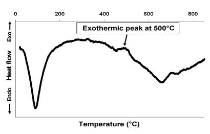
Figure 4. DTA curve of Mo-Mag<sub>001</sub>.
