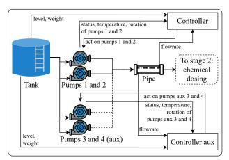
(c) A<sub>2</sub>: Design with an auxiliary controller and pumps, plus additional sensors.
