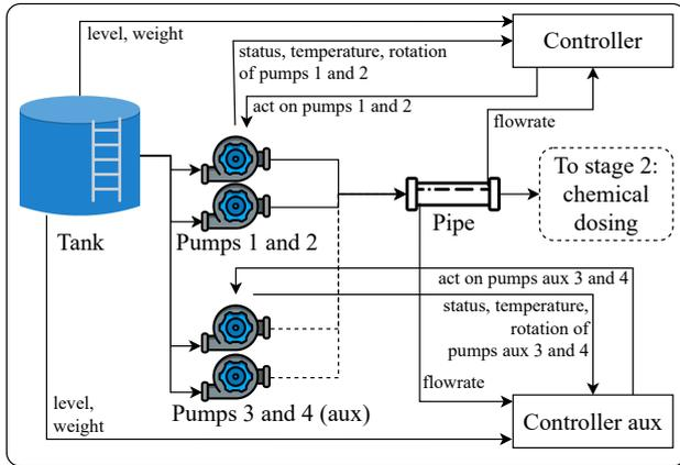
(c)  $A_2$ : Design with an auxiliary controller and pumps, plus additional sensors.
