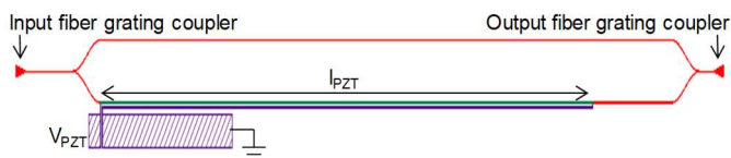
Fig. 1. Schematic view of a Mach-Zehnder interferometer, with the PZT actuator incorporated onto one of the arms above a straight waveguide, used to measure the efficiency of a thin-film PZT actuators as a stress-optic modulator.
