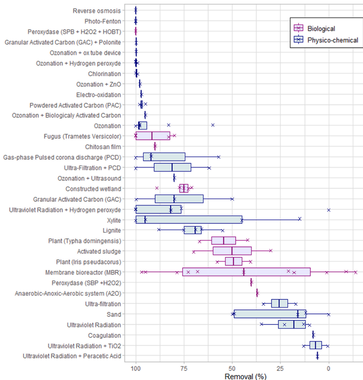
Fig. 4. Removal efficacy of furosemide by different advanced processes (%). Each x represents a value of furosemide removal. The purple boxes represent the techniques for which the removal of furosemide is done by a biological process and the blue boxes represent those for which the process is physicochemical (Machado et al., 2017; Nielsen et al., 2013; Vymazal et al., 2017; Park et al., 2017; Kovalova et al., 2012; Rostvall, 2017; Joannis-Cassan et al., 2021; Sandré et al., 2022; Almaqdi et al., 2019; Badia-Fabregat et al., 2016; Ajo et al., 2018; Jie, 2012; Rosal et al., 2010; Kjølholt et al., 2003a; Ibáñez et al., 2013a; Urriaga et al., 2013a; Klamerth et al., 2013a; Gómez et al., 2008a; Huerta-Fontela et al., 2011; Singh et al., 2015a; Ahmed et al., 2017; Arola et al., 2018; Cruz-Morató et al., 2014; Heidari et al., 2020; Ikonen et al., 2021; Kim et al., 2014; Kovalova et al., 2013; Llorens-Blanch et al., 2015; Machado et al., 2020; Muñoz et al., 2009; Reungoat et al., 2012; Rizzi et al., 2020; Verlicchi et al., 2015; Cuervo Lumbaque et al., 2020).
