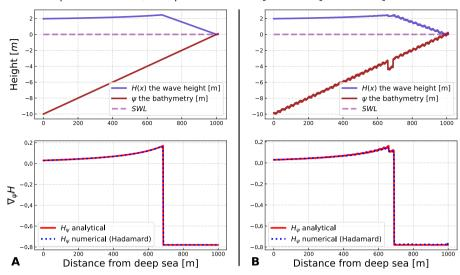
Figure 5: Comparison of numerical and analytical solution of  $\nabla_{\psi}H$  using Opti-Morph model. Configuration without (A) / with (B) perturbations,  $H_0 = 2$  m,  $h_0 = 10$  m and the wave period  $T_0 = 10$  s. In dodgerblue, the wave height H, in brown the bottom profile  $\psi$ , in red  $\nabla_{\psi}H$  calculated analytically, in blue  $\nabla_{\psi}H$  calculated by Hadamard strategy.
