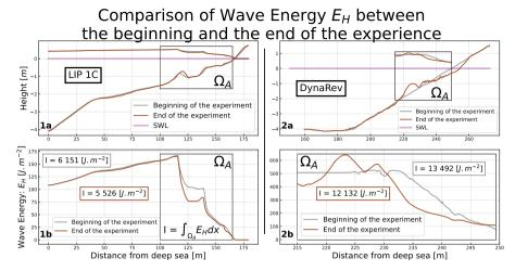
Figure 2: 1) LIP 1C experiment with H generated by XBeach. 2) DynaRev experiment with H measured by LIDAR. a) Bottom profile and averaged water height at the beginning of the experiment (grey), Bottom profile and averaged water height at the end of the experiment (brown). b) Wave energies associated with water heights. The energy is calculated on the black rectangle  $\Omega_A$ .
