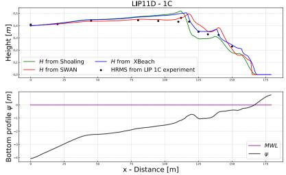
**Figure D3:** Wave results obtained with the Shoaling, SWAN and XBeach models. Sea bottom configuration from the LIP 1C channel experiment. Black points, measured HRMS, black bottom profile, green H from extended shoaling ( $H_{RMSE} = 0.045 \text{ m}$ ), red H from SWAN ( $H_{RMSE} = 0.033 \text{ m}$ ), blue H from XBeach ( $H_{RMSE} = 0.028 \text{ m}$ ).
