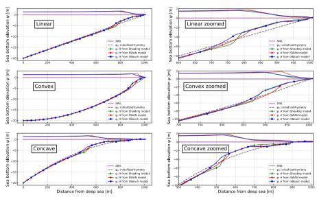
**Figure 9:** Evolution of  $\psi$  using Hadamard strategy with extended Shoaling (green), SWAN (red) and XBeach (blue) models. Simulation on open-sea configuration with linear, convex and concave configurations. Simulation parameters of  $H_0=2$  m,  $T_0=12$  s,  $h_0=20$  m,  $\Omega=1000$  m.
