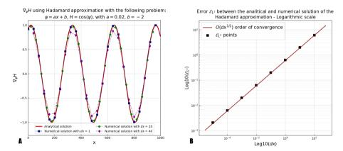
**Figure 4:** A) Calculation of  $\nabla_{\psi}H$  using Hadamard approximation with the following problem (see C.2):  $\psi = ax + b$ ,  $H = \cos(\psi)$ , with a = 0.02, b = -2. B) L2 error and order of convergence for a comparison between the analytical solution of the simple problem described in C.2 with  $H = \cos(\psi)$ .
