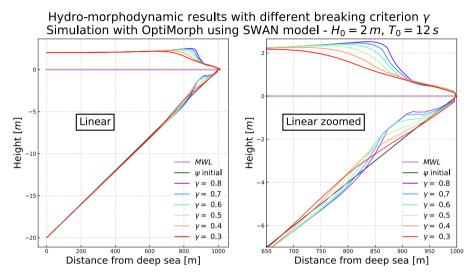
**Figure 11:** Hydro-morphodynamic results with different breaking criterion  $\gamma$  - Simulation with OptiMorph (Hadamard strategy) using SWAN model -  $H_0 = 2$  m,  $T_0 = 12$  s,  $h_0 = 20$  m.
