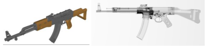
Fig. 6. 3D CAD model (left) and simulated X-ray projection (right) of a weapon.
