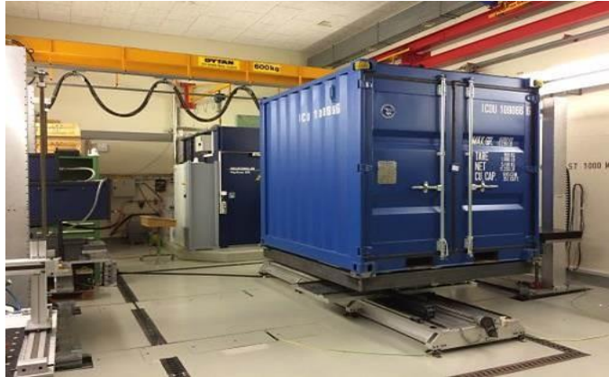
Fig. 1. ACXIS laboratory setup of cargo container imaged by linear accelerator (left) and new detector (right; hidden behind container).
