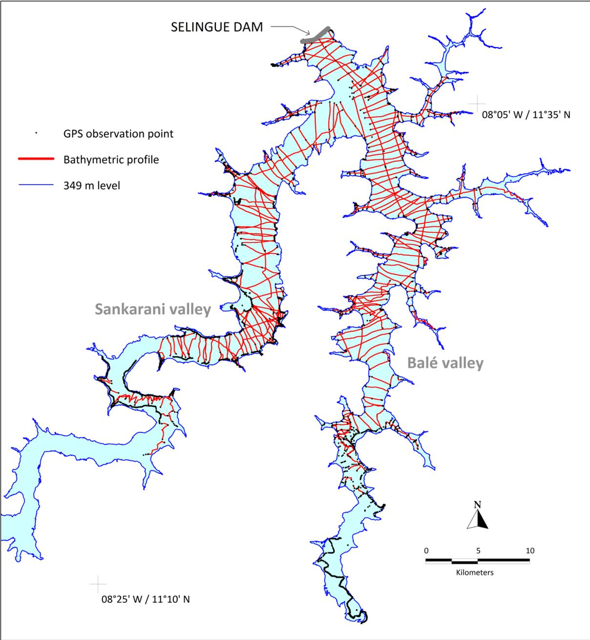
Figure 5: Topometry of Sélingué reservoir (IRD, 2008).
