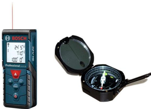
Figure 4. A portable laser distance measurer and geologic compass were used for the entire study method.
