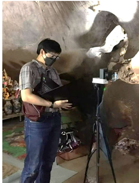
Figure 3. Cave profile scanning in the Muang-On show cave, Chiang Mai, Thailand. The equipment used exhibits the modified 2D LiDAR carefully attached to a camera tripod connected to a laptop. The LiDAR sensor rotates vertically to measure the distance between cave walls, floors, and roofs to create a single cave profile.
