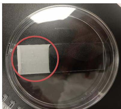
Figure 8. An illustration of a paint film with 22 nm nanoparticles, onto which 0.1 mL of bacterial suspension is spread, covered with a polypropylene film.
