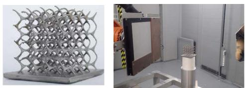
Figure 9: Lattice structure considered for the CT inspection (left) and view of the acquisition setup (right)
