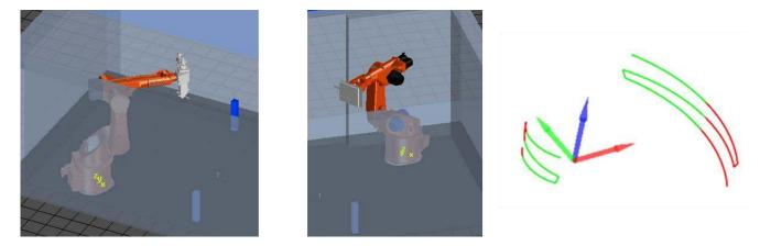
Figure 2: Model of the source robot (left) and the detector robot (centre) in CSR software and example of the visualization of the accessible trajectory (right).
