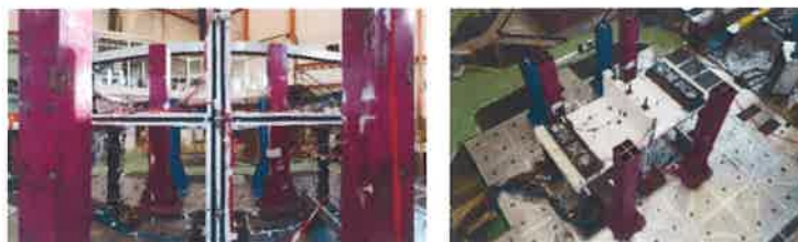
Figure 1. Front (left) and top (right) views of the mock-up mounted onto the "Azalée" shaking table (CEA/DEN)
