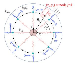
**Figure 5:** Reduction of components A and B into springs and mass connected on curved beams assembly ( $\rightarrow$ ) at screw nodes ( $\bullet$ ). Node positioning under deformed configuration with local displacements ( $u_j, v_j$ )
