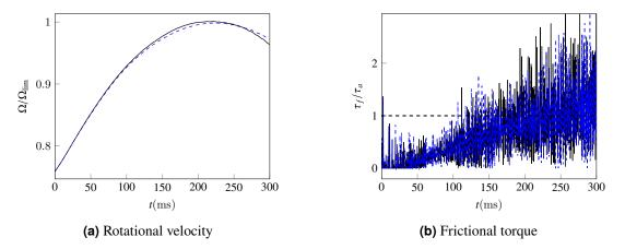
**Figure 7:** Transient response for the turbine rotation: 36 nodes (—) and 72 nodes (– ). Rotational velocity remains bounded since frictional torque overcomes aerodynamic torque.
