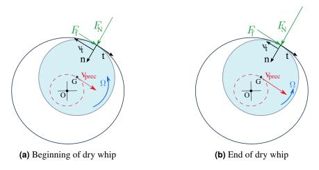
**Figure 16:** Description of velocities and efforts during a dry whip instability because friction force acts in the direction of vibration speed  $v_{prec}$  and opposed to rotational velocity  $\Omega$ .
