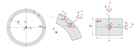
Figure 4: Stator geometry, reference frame and degrees-of-freedom for a curved Bernoulli beam
