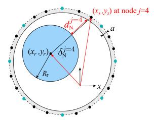
**Figure 6:** Computation of the nodal distance between de rotor center and the 4<sup>th</sup> node on the stator (j = 4)
