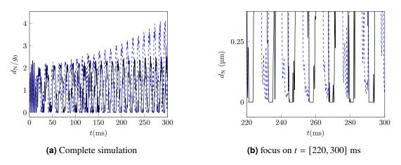
**Figure 25:** Gap function at node 17:  $\alpha = 0$  (—) and  $\alpha = 1.05 \times 10^{-5} \text{ K}^{-1}$  (--)
