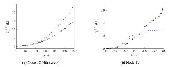
**Figure 24:** Energy source provided locally to stator nodes by friction, increases for any screw node with thermal dilatation, while it decreases for other nodes:  $\alpha = 0$  (—) and  $\alpha = 1.05 \times 10^{-5}$  K<sup>-1</sup> (--).
