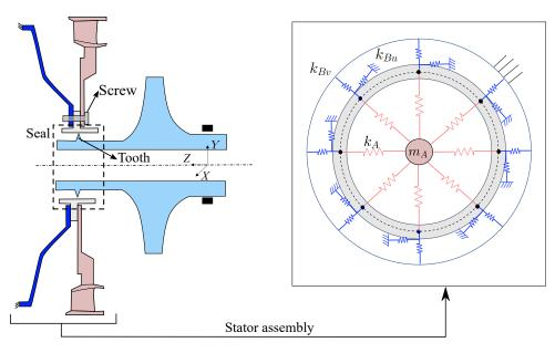
**Figure 2:** Rotor-stator system between static assembly and the turbine  $(\square)$  supported by a rear bearing  $(\square)$ . Simplification of the assembly ring  $(\square)$ , component A  $(\square)$  and component B  $(\square)$  into a ring supported by equivalent springs located at screw points.
