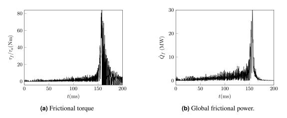
**Figure 14:** Dynamical response for  $\mu = 0.15$  and  $N_e = 36$ .
