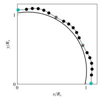
**Figure 26:** Rotor-Stator contact interface with thermal dilatation at the end of simulation t = 300 ms for a 90°-sector: Rotor rigid disc (—), stator deformed shape (-), contact points (×) and screws (). Amplitudes are magnified by a scale factor 5 for illustration purposes. Blue points represent screw nodes and black ones, conventional nodes. A node marked with a cross indicates closed contact.
