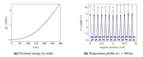
**Figure 10:** Thermal response: 36 nodes (—), 72 nodes (--). Total frictional energy is identical with mesh refinement but temperature disctibution shows extremely local peaks at screw nodes.
