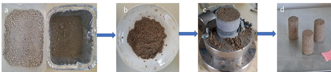
Figure 2. Sand and binder (a), sample preparation (b), manufacturing of samples (c) and cylindrical samples (d).
