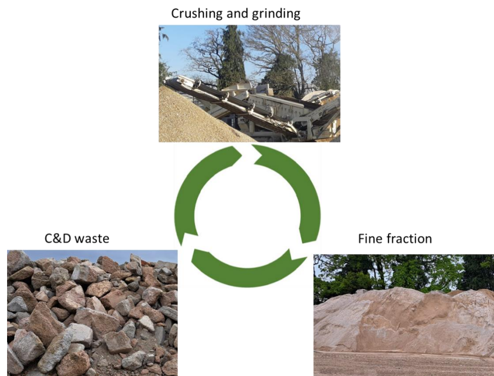
Figure 1. Transformation of CDW waste into coarse and fine aggregates.
