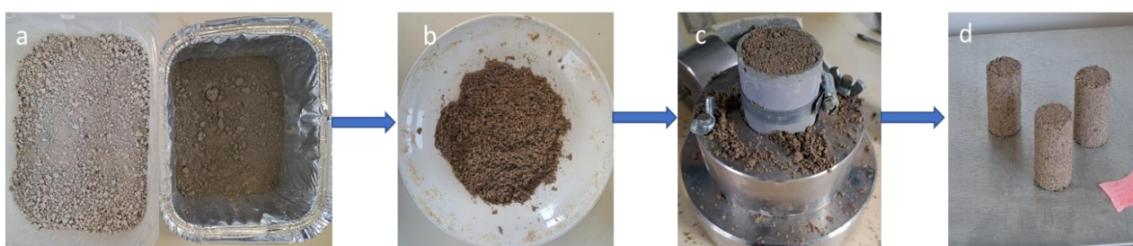
Figure 2. Sand and binder (a), sample preparation (b), manufacturing of samples (c) and cylindrical samples (d).
