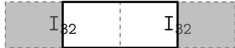
(a) Fetching the bottom half of a 32-bit instruction and the top half of another 32-bit instruction.
