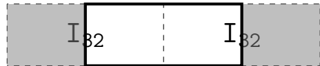
(a) Fetching the bottom half of a 32-bit instruction and the top half of another 32-bit instruction.
