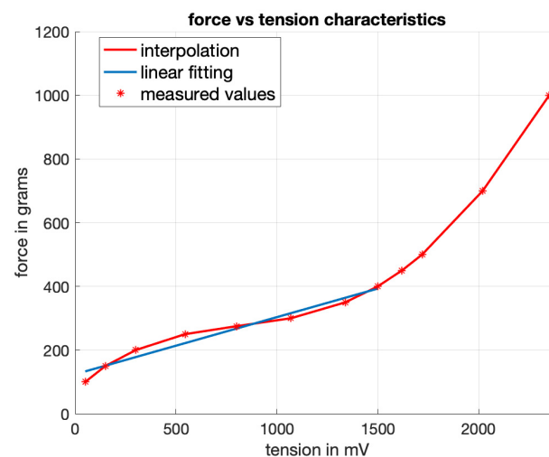
Figure 2. Static force in grams is related by a linear function (blue line) to tension output in the range from 50 mV to 1500 mV.
