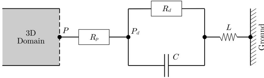
Figure 6: Representation of the four components Windkessel model.
