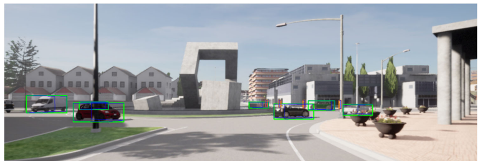
Fig. 2 Bounding boxes for cars and pedestrians with their two lower points on the ground as given from our Dataset built from CARLA. The green frame represents the 2D bounding boxes extracted from the 3-Dimensional (3D) bounding boxes (in blue) given by the simulator
