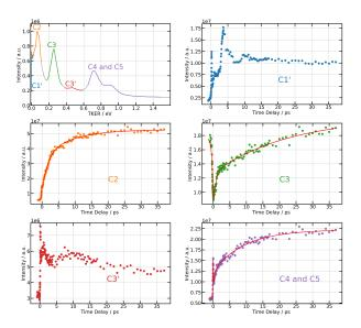
Fig. 6 269/807 nm experiment *Top left panel*: TKER spectrum obtained by integrating  $S_0^{cation}(KER,\tau)$  along the KER axis (vertical axis in Fig 5. The colours and labels C1', C2, C3, C3', C4 and C5 isolate 6 regions of interest (ROI). Note that TKER is twice the I<sup>+</sup>KER shown Fig.5. *Other panels*: time dependencies of the signal associated with each ROI. Dots show the experiment. Solid lines in ROIs C2, C3, and C4,5 are fit using the time constants listed in Tab.1.
