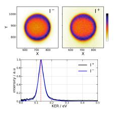
Fig. 2 Pump only experiment at 269 nm Raw VMI images of I $^-$  (top left panel) and I $^+$  (top right panel) and kinetic energy release (KER) (bottom panel) for each ion. The red dashed line in the bottom panel is the expected KER energy from energy conservation. The colour scale for intensities in the I $^-$  and I $^+$  images is shown at the right hand side of the figure.
