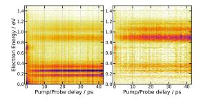
Fig. 7  $\frac{269/807 \text{ nm experiment}}{(E,\tau)}$  3D-plot of the fs-TRPES signals  $S_0^{elec}(E,\tau)$  (left panel, isotropically distributed photoelectrons) and  $S_2^{elec}(E,\tau)$  (right panel, polarised electrons) with the same colour map as in Fig. 3.
