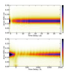
Fig. 3 \_269/807 nm experiment - 3D-plot of the fs-TRKERS signal  $S_0^{anion}(\text{KER},\tau)$ , up to 40 ps (top panel) and 2 ps (bottom panel): the signal intensity is given by the colour map shown at the right hand side of the figure; it is plotted as a function of the I<sup>-</sup> KER energy (vertical axis in eV) and pump-probe delay (horizontal axis).
