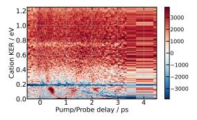
Fig. 11 266/334 nm experiment 3D-picture of  $S_2^{cation}(E,\tau)$  using the colour scale shown at the right hand side of the figure. Positive values indicate preferential dissociation along the polarisation direction of the pump laser.
