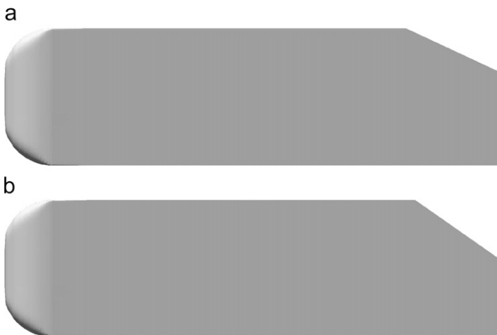
Fig. 1. Ahmed body view: (a) 25^\circ rear slant; (b) 35^\circ rear slant.
