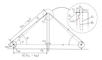
Figure 15. Schematic of the pulley system for the loading tests.
