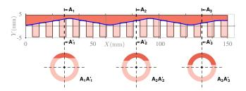
**Figure 4.** Rod with continuously variable sections (dark red), equivalent to a tube with variable notches (light and dark red). Top: in red: longitudinal section (or profile) of the tube; in blue: interpolation of the tube depth profile with equation (1). Bottom: for any value of the continuous label X, the blue function can be evaluated, yielding the continuous U-shaped cross-sections along the equivalent rod. See also Extension 2.
