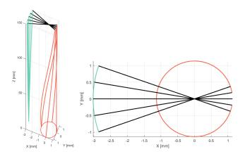
**Figure 21.** 2-tube CPPR actuated in rotation only. Perspective view (left). Top view (right). The red arc of circle represents the path taken by the centroid of tube 2 at the base of the CPPR, while the green arc of circle represents the path taken by the centroid of tube 1 at the top of the CPPR. The solid black line represents the rigid segment connecting the centroids of the two tubes at the tip of the CPPR. Their intersection lies on the central axis of the CPPR.
