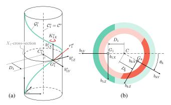
**Figure 10.** (a) Perspective view of one tube (number 1) in the resting configuration of the CPPR. In red are indicated the offset twists due to design. (b): Section view of the leader tube (numbered 1) and a follower (numbered k) in a CPPR able to deform in 3D. Tube k can rotate of an angle  $\theta_k$ , with respect to tube 1 around the centerline of the CPPR. Note that this figure generalizes the planar context of Figure 8(c) where we had  $\theta_k = 0$ .
