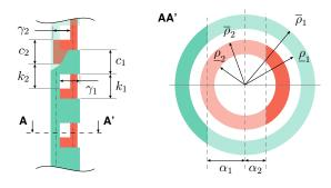
**Figure 3.** Longitudinal and radial design parameters of notches of tubes 1 and 2, displayed on a partial front (left) and sectional view (right) of a CPPR. Remind that  $\gamma_i$  and  $\alpha_i$  are related by  $\gamma_i = \overline{\rho}_i + \alpha_i$ .
