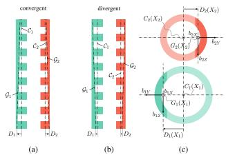
**Figure 6.** Varying the depth of the notches along the tubes varies the position of their offset centroid line. (a,b) Tubes with convergent (divergent) centroid lines. The notch depth linearly decreases (increases) towards the tip of the CPPR. (c) Cross-sectional frames and centroid offsets of the inner (top) and outer (bottom) tubes.
