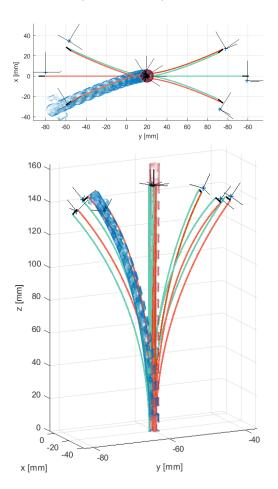
**Figure 24.** 3D shape measurements of a 2-tube CPPR (prototype  $\mathcal{R}_1$ ) actuated in translation and rotation. The frames at the tip of the snapshots are defined by pose measurements. The thick red and green lines are the simulated centroid lines of the tubes.
