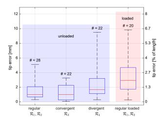
**Figure 17.** Boxplots of the tip position error between experimental results and simulations for all tests. The first three groups are unloaded cases  $(f_+=0)$ . The  $\sharp$  symbol is related to the number of experiments.
