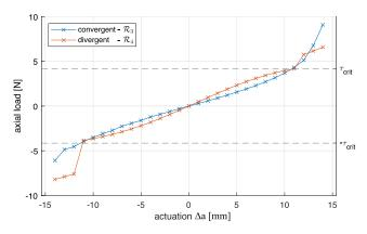
**Figure 25.** Axial load in the variable centroid line prototypes. The absolute value of the load increases with increasing actuation translation. Beyond  $|\Delta a| > 11 \, \mathrm{mm}$  the axial load was found to exceed Euler's critical load of the rods composing the CPPRs.
