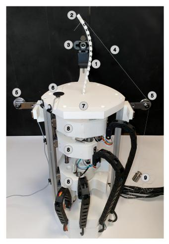
**Figure 11.** Multi-stage CPPR actuation unit with a mounted prototype used for experimental validation. In the experiments presented in this paper, only one stage was used to translate one CPPR tube with respect to the other. (1) CPPR; (2) tip electromagnetic sensor; (3) camera; (4) nylon thread; (5) idler deflection pulleys; (6) reference electromagnetic sensor; (7) baseplate; (8) translation stages; (9) calibration weight.
