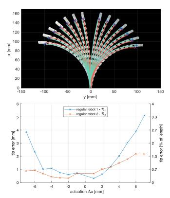
Figure 12. Top, snapshots of the experiments and simulation results for the regularly notched prototypes, here with prototype  $\mathcal{R}_1$ . The colored lines represent for each case the centroid line of tube 1 and 2, respectively, with corresponding colors. The blue marks are the tip EM sensor data. The purple marks are the simulated robot tips. Bottom, tip error as function of the actuation  $\Delta a$  for both regularly notched prototypes. See also Extension 6.
