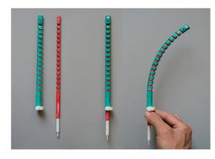
**Figure 1.** Photo of an archetypal two-tube CPPR. From left to right: The outer and inner notched tubes separately. The CPPR with its tubes nested together, at rest, and bent under the effect of a pulling force applied to the tip of the inner tube. Observe how the tubes slide coaxially in relation to each other.
