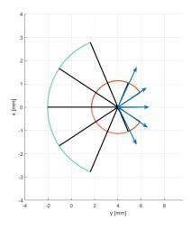
**Figure 23.** Top-view of the 2-tube CPPR  $(\mathcal{R}_1)$  actuated in rotation only with  $\Delta\theta_d \in \{-\pi, -\pi/2, 0, \pi/2, \pi\}$  rad. The blue arrows represent one of the base vectors of the frame of reference attached to the tip of the CPPR and measured by the Aurora sensing device. The values of  $G_1$  and  $G_2$  are calibrated and the corresponding vectors of the model (black solid lines) are shown.
