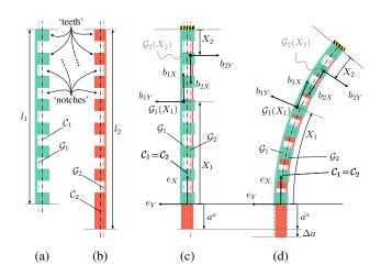
**Figure 2.** Composition, working principle and frames of a CPPR. Outer (a) and inner (b) tubes at rest with their centroid and centerlines. The assembled tubes, forming the CPPR in a resting configuration, with the cross-sectional frames attached to the tubes (c). Actuating the CPPR with  $\Delta a > 0$ , bends it in a deformed configuration and makes the frames move (d).
