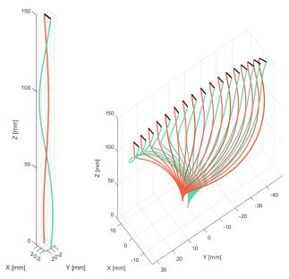
**Figure 22.** 2-tube CPPR with helicoidal centroid lines actuated in translation. (left) Configuration at rest. (right) Snapshots of a deformation due to a translation of tube 2 from  $-10 \,\mathrm{mm}$  to  $10 \,\mathrm{mm}$ .
