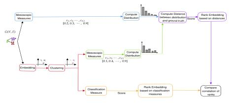
Figure 1: Flowchart of the experimental setup to evaluate the performance of the network embedding algorithms. Mesoscopic metrics are calculated individually for each of the network's communities.
