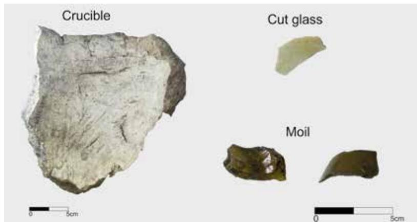
Fig. 7. Production remains in the Workshop C/E-93 (photo and image by S. Berrica).
