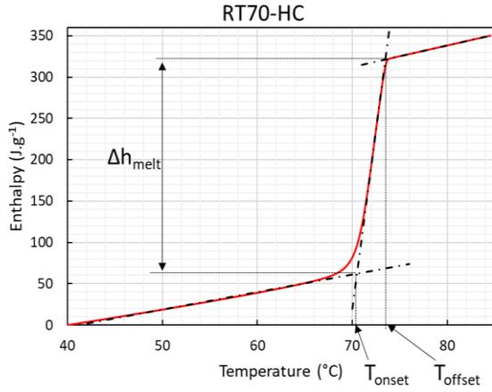
Fig. 2. Specific heat of the RT70-HC (calorimetry)
