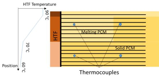
Fig. 7. Influence of the upstream PCM melt on the downstream heat flux
