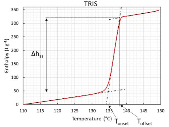
Fig. 3. Specific heat of the TRIS (calorimetry)
