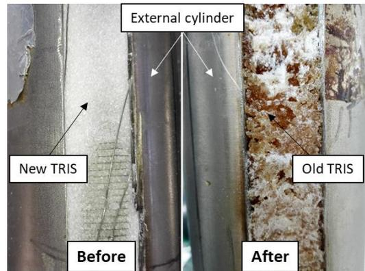
Fig. 18. TRIS before and after five thermal cycles
