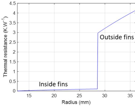
Fig. 11. Thermal resistance with and without aluminum fins
