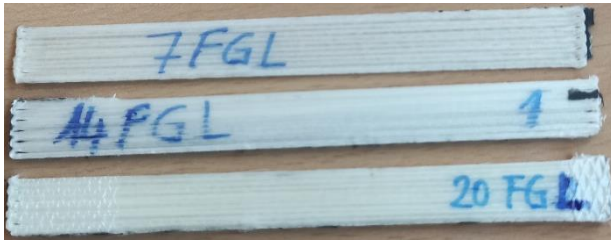
Figure 7: 3D printed glass fiber samples.
