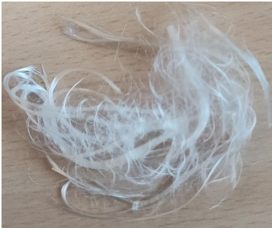
Figure 9: 3D printed glass fibers after acid digestion of nylon and other constituents.
