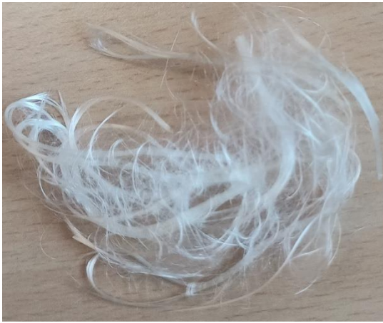
Figure 9: 3D printed glass fibers after acid digestion of nylon and other constituents.
