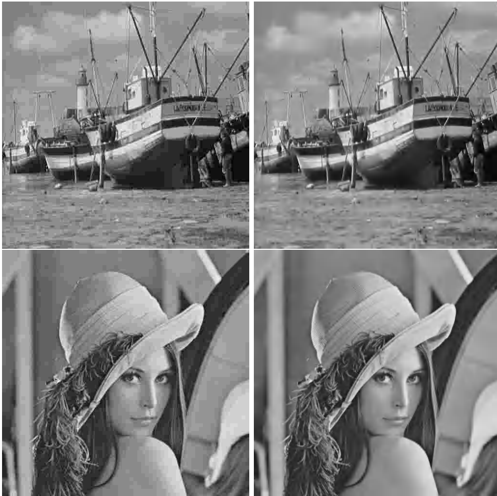
FIGURE 33 – Examples showing the difference in image quality when using the same compression rate of 0.2 bpp, either with the JPEG standard on the left or JPEG2000 on the right. It can be observed that at higher compression rates, the use of wavelets allows capturing redundancies at all scales to achieve better image reconstruction.
