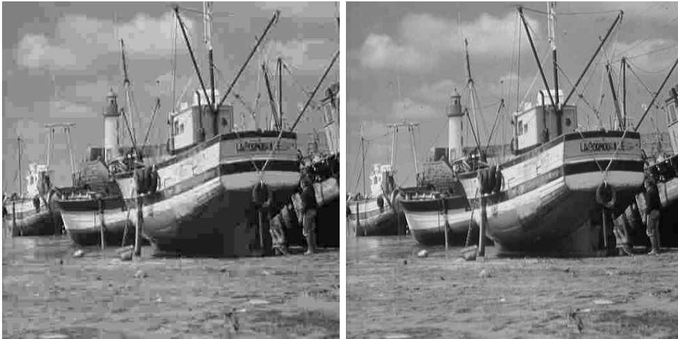
FIGURE 31 – Left: JPEG compression rate is 0.2 bpp. Right: JPEG compression rate is 0.5 bpp.
