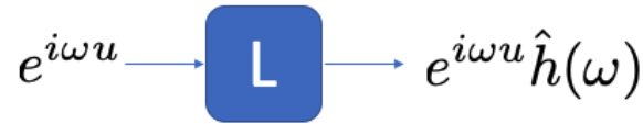
FIGURE 13 – The linear operator covariant under translation, denoted as L , has exponential functions e^{i\omega u} as its eigenvectors, with associated eigenvalues equal to the values of its estimated Transfer Function at \omega (cf. \hat{h}(\omega) ).
