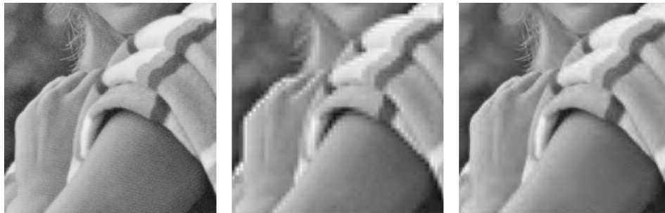
FIGURE 56 – Inset of an original 512 \times 512 image, in the middle a linear approximation that reduces the image size by a factor of 16, and on the right, a non-linear approximation also with 1/16 of the initial coefficients, starting from a decomposition that reduces by a factor of 32 and complements with detail coefficients.
