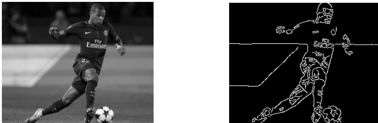
FIGURE 9 – Illustration of the use of "classical" image structure analysis techniques: here, edge detection.
