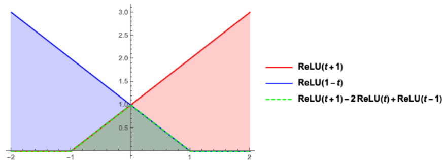
FIGURE 49 – With a linear combination of ReLU, we can obtain a "triangle" function (in green).
